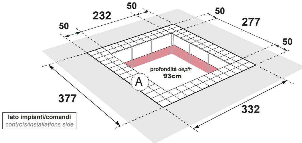
A DETTAGLI VANO INCASSO INSPECTION COMPARTMENT DETAILS
